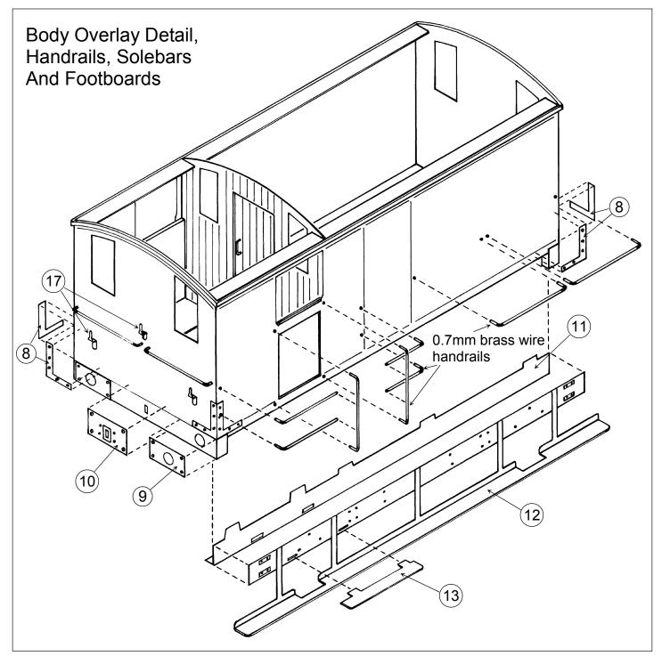
3. I now find that it is best to detail up the body as far as possible before fitting the solebars/ footboards as these can be a little vulnerable to getting bent as you work.
