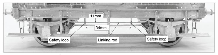
Using 0.7mm brass wire form up a rod to link the inner brake yokes and solder into position so that it runs parallel to and 11mm below the wagon floor. Again using 0.7mm brass wire form up two safety loops for this rod and solder to the underside of the floor 34mm apart. The centre footboard support will give a good visual guide for the vans centre line.
