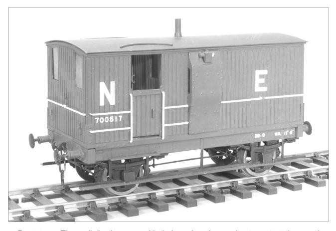
**Prototype.** These distinctive vans with their enclosed verandas to protect the guard from the worst of the Scottish weather were built in the early 1920s by the NBR to diagram 32B. They spent most of their working lives in LNER livery but a few continued in service with British Railways.
